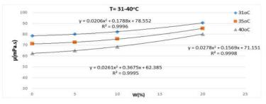
Figure 5 – Crude oil viscosity vs water saturation under temperatures of 31-40oC 31-40°C
